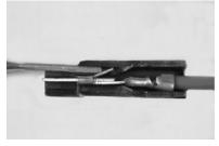
DETAIL "A" Each terminal has a locking "tang" to lock it into the connector. This tang must be collapsed by using a very thin screwdriver or pick in order to remove the terminal and wire from the connector.
